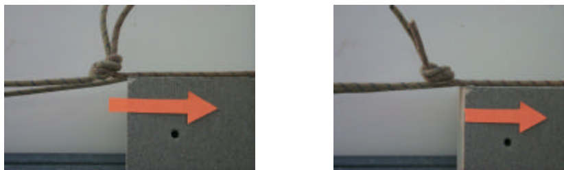
(a) Tails leading (b) Tails trailing Knot tails on the reverse edge. The arrow indicates the direction of pull.
