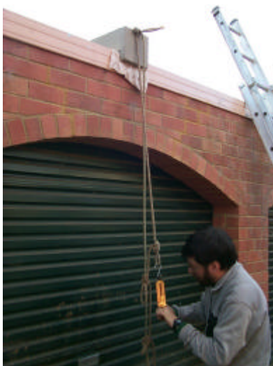
(a) The author using a spring balance to measure the load when pulling a knot over a 90° edge at his garage.
