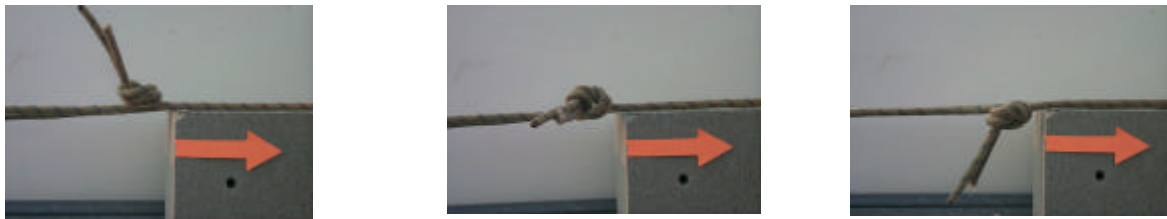
(a) Tails up Knot tails on the reverse edge. The arrow indicates the direction of pull. (b) Tails level (c) Tails down Figure 13
