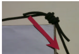
The Double Fisherman's Knot jamming on the edge. The arrow indicates the direction of pull. Figure 8
