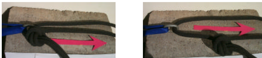
(a) The Overhand knot against the sling (b) away from the sling The arrow indicates the direction of pull.
